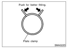
After installing leaf spring clamps, apply force to them in the direction of the arrow, tightening rubber hose equally all around.
